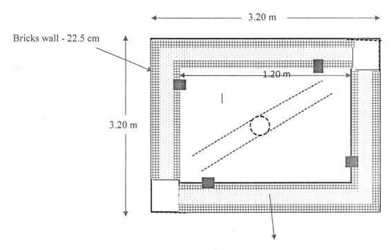
Prefabricated perforated base - 50 cm width
