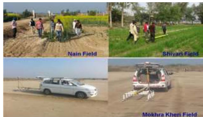
Fig.1. Manual and cart surveys with DUALEM-21 and GPS instruments at three sites
