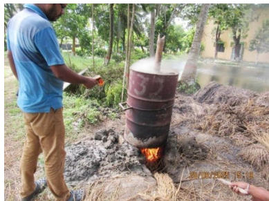
Measuring temperature using an infrared thermometer while biochar preparation
