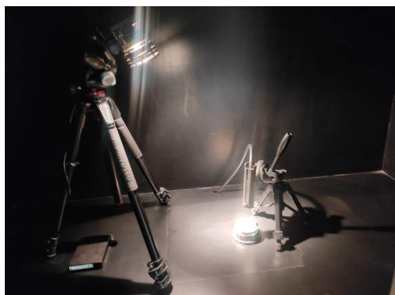
Fig 2.7 SVC 1024i spectroradiometer setup for generating VNIR spectra of soil samples
