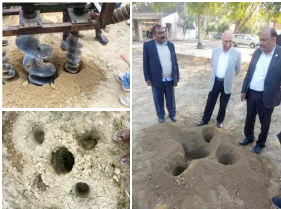
Holes made in sodic soil by multiple auger system
