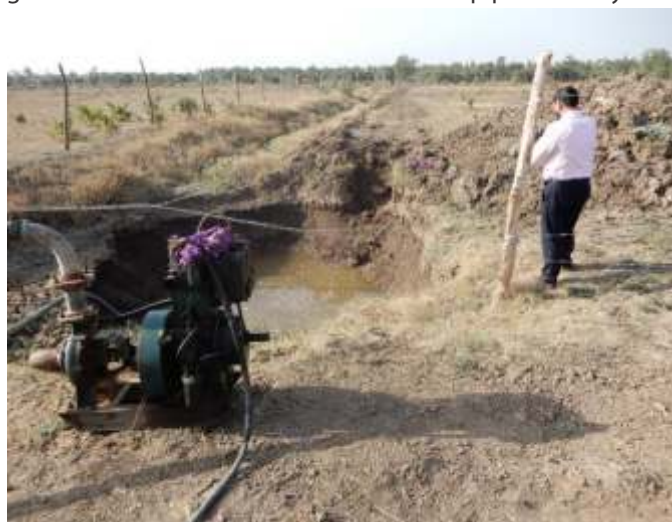
Field condition of a pilot SSD system for salt leaching and a temporary storage sump well filled with drainage effluent water from the SSD system
