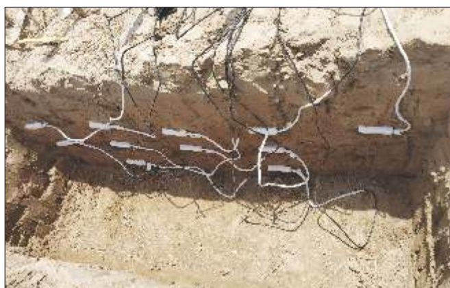
Horizontal and vertical GS3 soil water and salinity sensors at Nain Farm, Panipat
