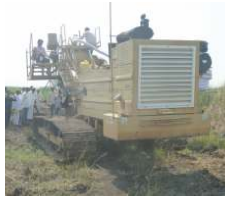
Implementation of SSD projects using small trenchers in Maharashtra and Karnataka and their monitoring
