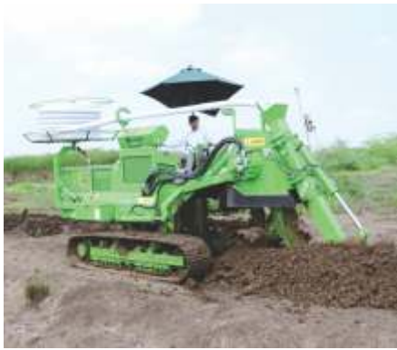
Implementation of SSD projects using small trenchers in Maharashtra and Karnataka and their monitoring
